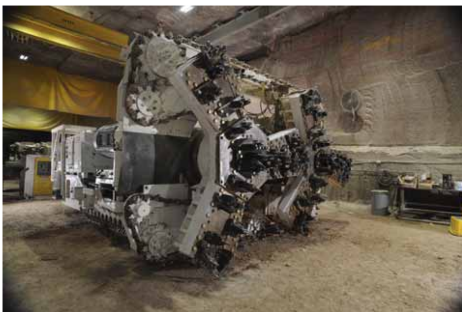
Figure 1. Underground continuous mining machine. Courtesy of Prairie Machines and Parts Ltd (PMP).
