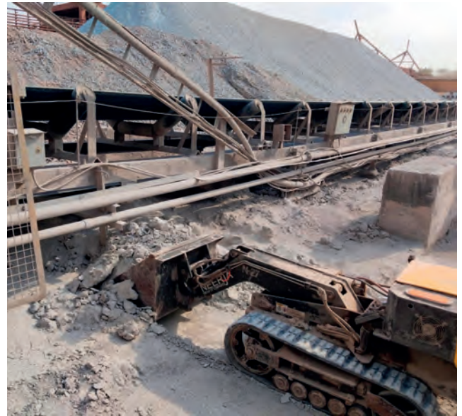
Figure 3. A 69 cm wide mini-loader cleaning under a conveyor.
