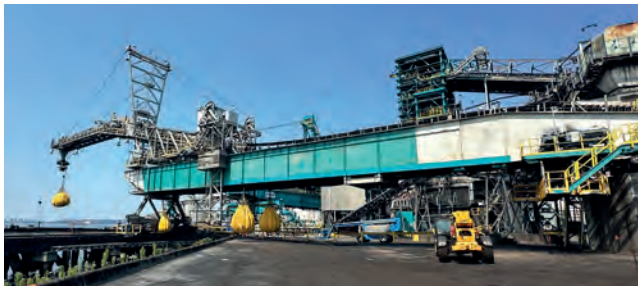
Figure 3. Final government-regulated load testing of a radial ship loader after a head chute replacement project, Canada.
