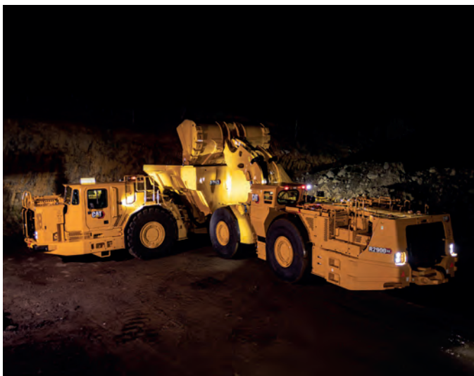
Figure 2. The R2900 XE offers 35% improved breakout force over the R2900G and delivers a three to four-pass match to the Cat AD63 truck.
