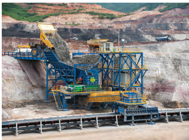
Figure 2. A Sizer Station with dual tipping points processes overburden quickly and keeps the operation moving smoothly.
