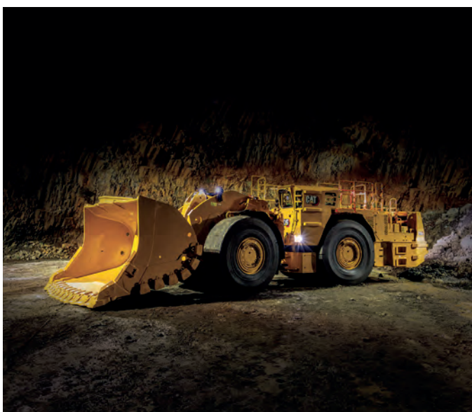
Figure 1. The Cat R2900 XE employs a high efficiency electric drive system and is powered by the quiet and reliable Cat C15 engine.
