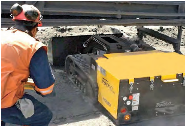
Figure 1. A 122 cm wide mini-loader manoeuvres effortlessly beneath low-clearance mining conveyor.
